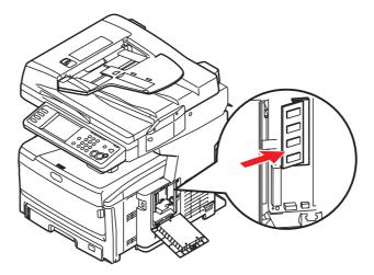
**7.** Gently push the board into the RAM expansion slot until it latches in and will not go any further.
